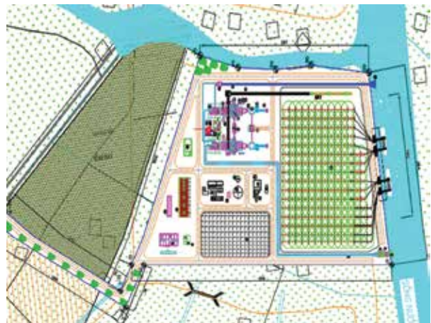
Layout of Hau Giang Biomass Power Plant
